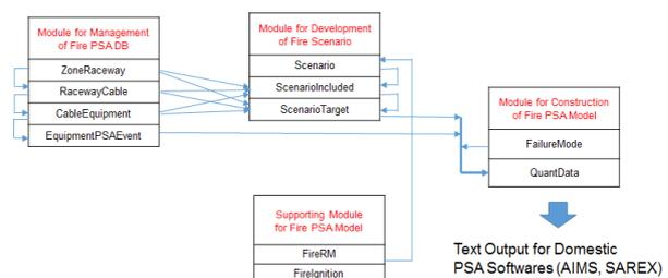
Fig. 2 Relation between the modules for the ProFire-PSA
