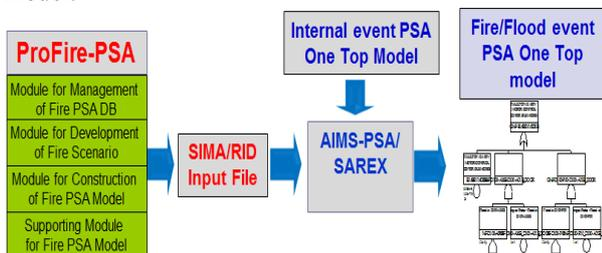
Fig. 1 Relation between the ProFire-PSA and AIMS-PSA/SAREX
