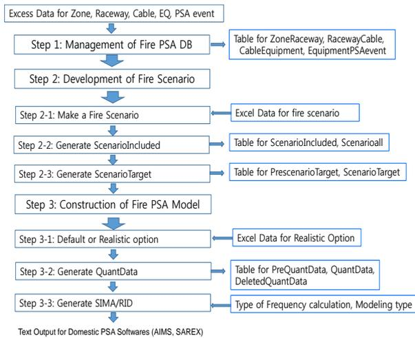
Fig. 3 Execution process of the ProFire-PSA
