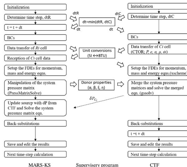
Fig. 1. Schematic diagram of the modified calculation logic of MARS-KS and CTF code coupling [4].
