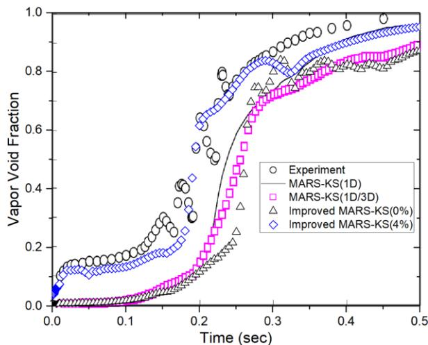
Fig. 11. Void fraction comparison at vessel channel 8.
