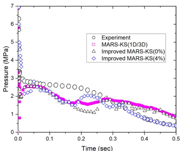
Fig. 10. Pressure comparison at vessel channel 8.
