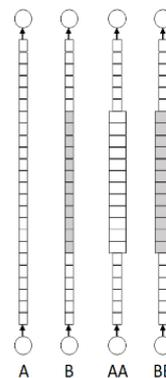
Fig. 2. Nodalization of the vertical pipe test.
