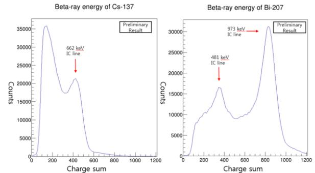
Fig. 4. The beta-ray energy spectra of  $^{137}\text{Cs}$  (left) and  $^{207}\text{Bi}$  (right) sources. The x-axis is the area (charge quantity) of the signal.
