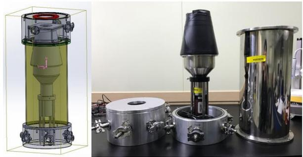
Fig. 1. The beta-coincidence spectroscopy.
