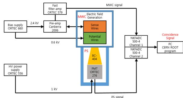
Fig. 2. The schematic diagram of the BCS measurement system.
