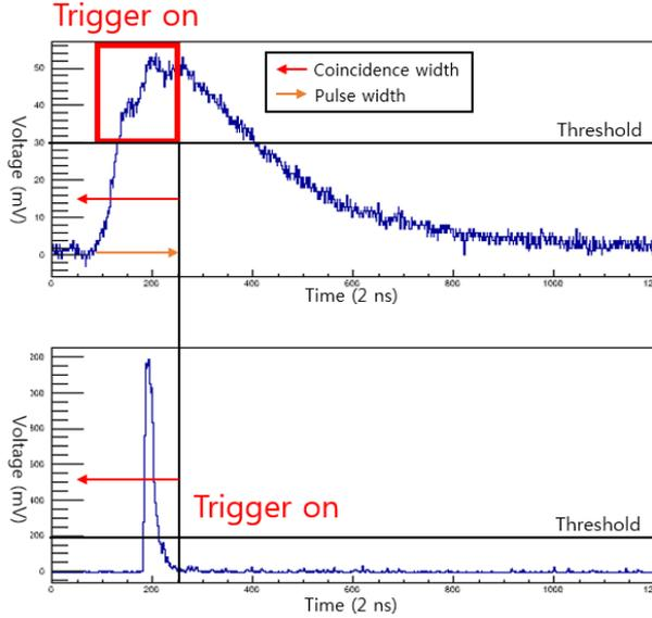
Fig. 3. Selecting process of coincidence signal.
