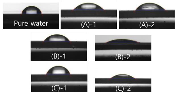
Fig. 5. Images of contact angle for heaters tested with pure water, (A) amorphous particles, (B) porous particles with 2nm of pore, (C) porous particles with 4nm of pore in (1) 0.1ppmv and (2) 10ppmv of concentration region
