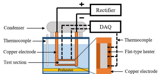
Fig. 2. Experimental apparatus for pool boiling test
