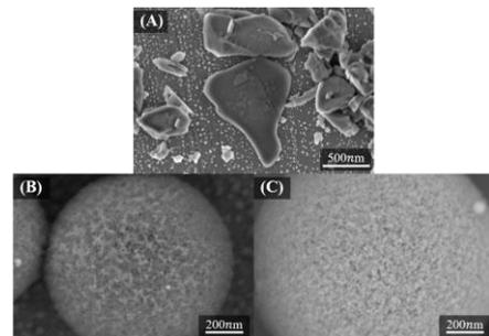
Fig. 3. Images of (A) amorphous and porous silica particles with pores of (B) 2nm and (C) 4nm
