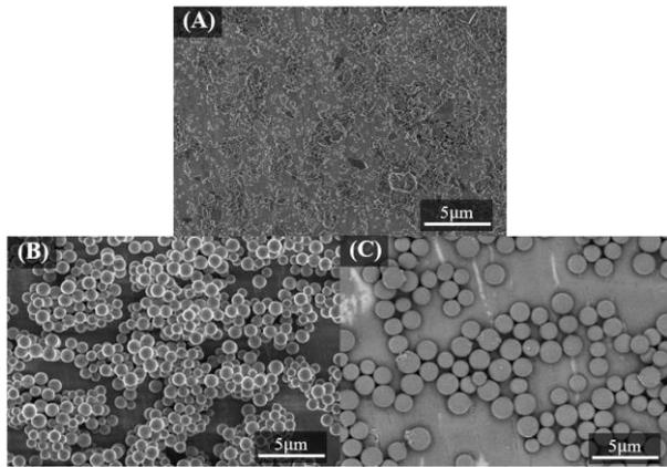
Fig. 6. SEM images of heater surface after experiments with suspension in 10ppmv of concentration((A): Amorphous particles, (B): Porous particles with 2nm of pore, (C): Porous particles with 4nm of pore)
