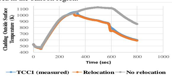
Figure 2: Cladding outside surface temperature variation with time.
