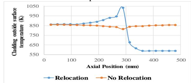
Figure 4: Calculated cladding outside surface temperature versus axial position at 800sec.
