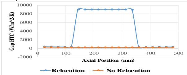
Figure 8: Gap heat transfer coefficient (HTC) along the fuel rod during the rupture time of 315.5 sec.
