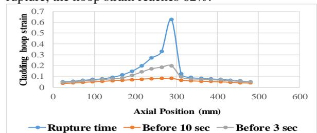
Figure 6: Cladding hoop strain values along the fuel rod up to the time of cladding rupture (315.5 sec).
