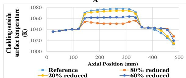
Figure 10: Cladding outside temperature along the fuel rod at rupture time of 315.5 sec: A. Packing fraction impact, B. Thermal conductivity impact.
