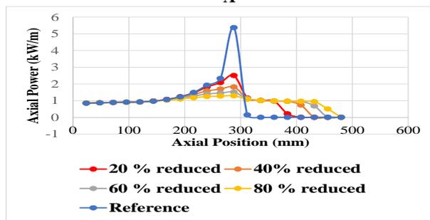
Figure 11: Variation of axial power along the fuel rod at rupture time of 315.5 sec. **A.** Packing fraction impact, **B.** Thermal conductivity impact.
