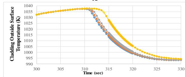
Figure 9: The influence of packing fraction (A) and crumble thermal conductivity (B) on cladding temperature with time.
