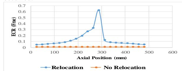
Figure 5: Equivalent cladding reacted (ECR) versus axial position at the rupture time of 315.5 sec.
