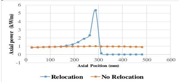
Figure 7: Axial power versus axial position at rupture time of 315.5 sec.
