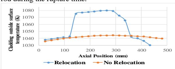
Figure 3: Cladding outside surface temperature versus fuel axial position during rupture at 315.5 sec.
