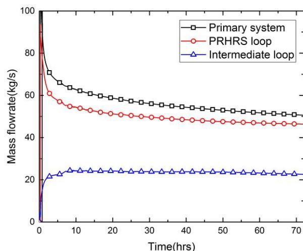
Fig 3. Mass flowrates in primary system, PRHRS loop, and intermediate loop.
