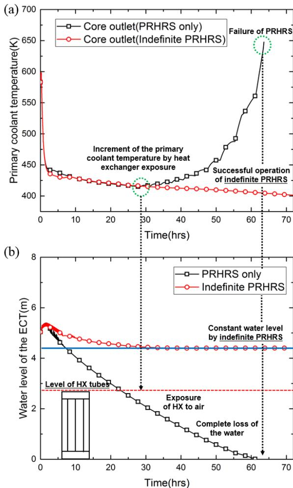
Fig 5. Comparison simulations for the cases with PRHS only and indefinite PRHS. (a) Change of primary coolant temperature, (b) Change of water level.
