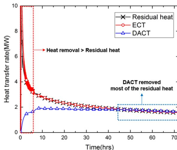
Fig 4. The change of residual heat and heat transfer rate of ECT and DACT.
