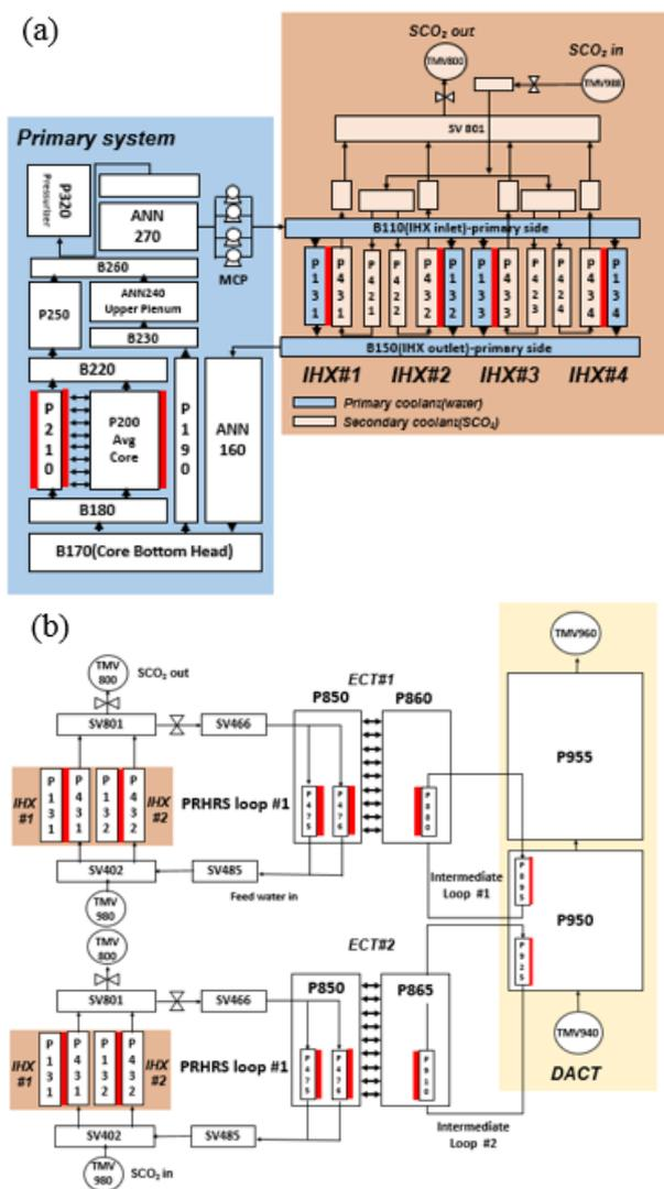
Fig 2. MARS-KS modeling (a) Primary and Secondary system of ATOM, (b) Indefinite PRHRS
