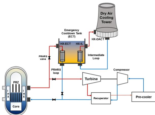
Fig. 1. Schematic diagram of indefinite PRHRS at ATOM
