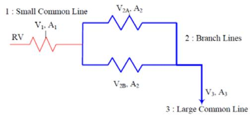
Fig. 3. Branch Flow Model for RVCH Vent Path
