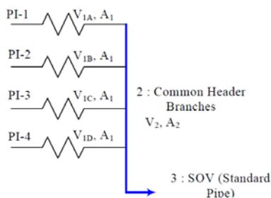
Fig. 2. Branch Flow Split Model for PZR Vent Path
