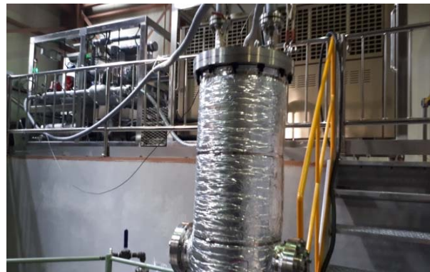
Fig. 1. Forced Circulation Drying Test Equipment
