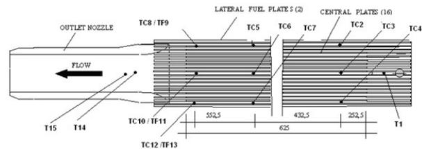
Fig. 5 Measurement Location of Temperatures
