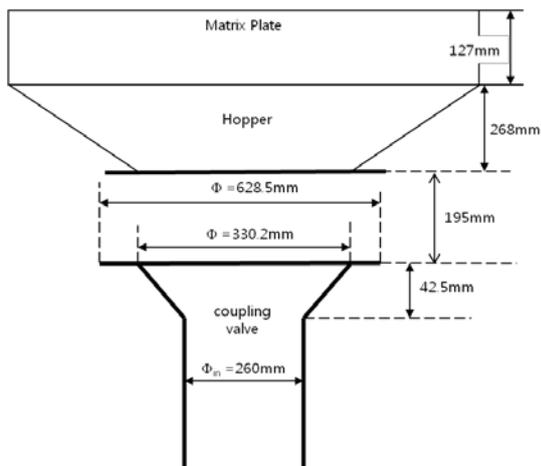
Fig. 3 Schematic Diagram of the Coupling Valve
