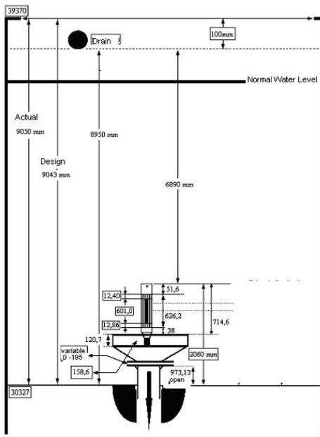
Fig. 2 Schematic Diagram of the Reactor Pool and Structure
