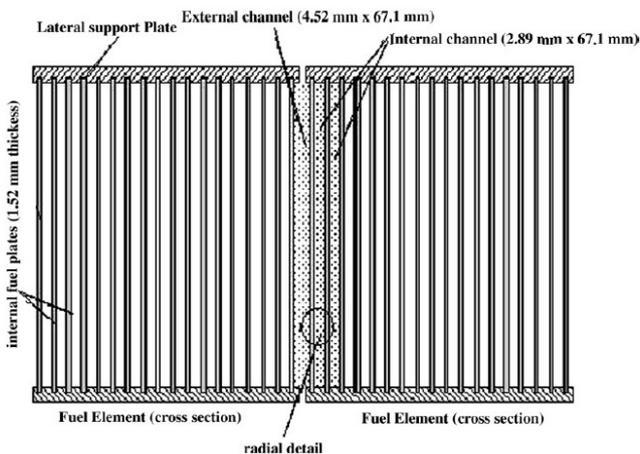
Fig. 4 Cross Section of Two Fuel Assemblies
