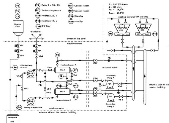
Fig. 1 Schematic Diagram of the Reactor Cooling System
