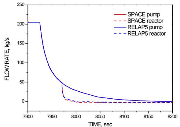
Fig. 7 Mass Flow Rate of Reactor and Pump
