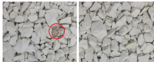
Figure 2. Sample Image of NaP Zeolite Dataset (Left: Defect Included, Right: Normal NaP Zeolite)
