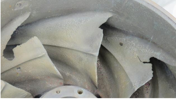
Fig. 3. Serious comprehensive damage of erosion such as pitting on the surface and sharp cross section of the impeller vane.
