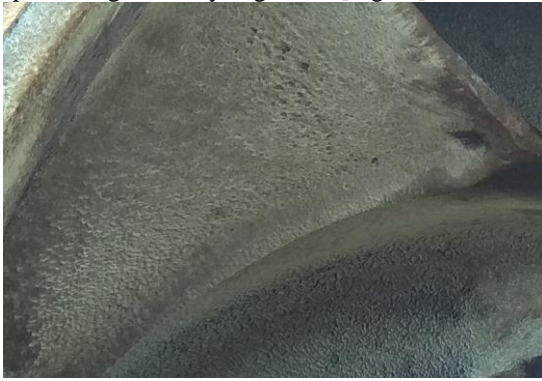
Fig. 7. Al-bronze impeller surface with cavitation pitting after 3.5 years operating without performance degradation and significant vane pass frequency peak.
