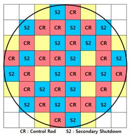
Fig. 2 Reactor Core Arrangement of for BANDI-60S
