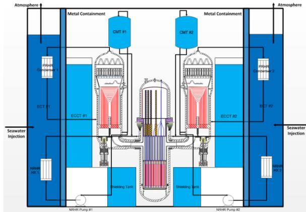
Fig. 3. Basic Concept of the Passive Safety Systems
