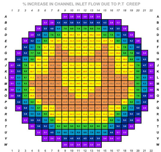
Fig. 2. % increase on channel flows due to PT creep
