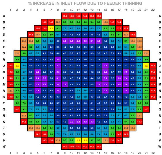
Fig. 3. Increase in channel flows due to feeder thinning
