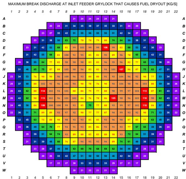
Fig. 7. Maximum break discharge at inlet feeder gray-lock that causes fuel dry-out [kg/s]
