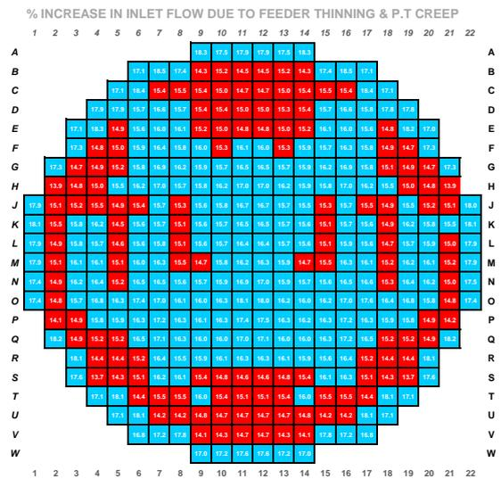
Fig. 4. Increase on channel flows due to feeder thinning as well as pressure tube creep
