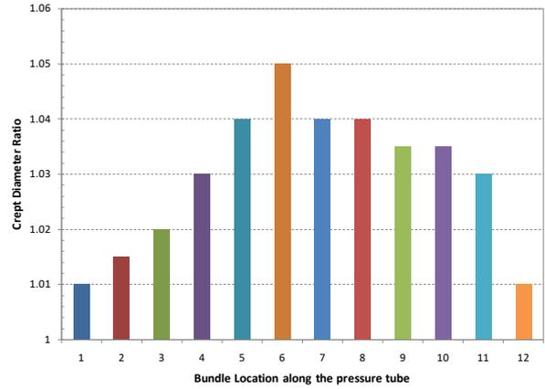
Fig. 1. Diametrical creep profile used in the analysis
