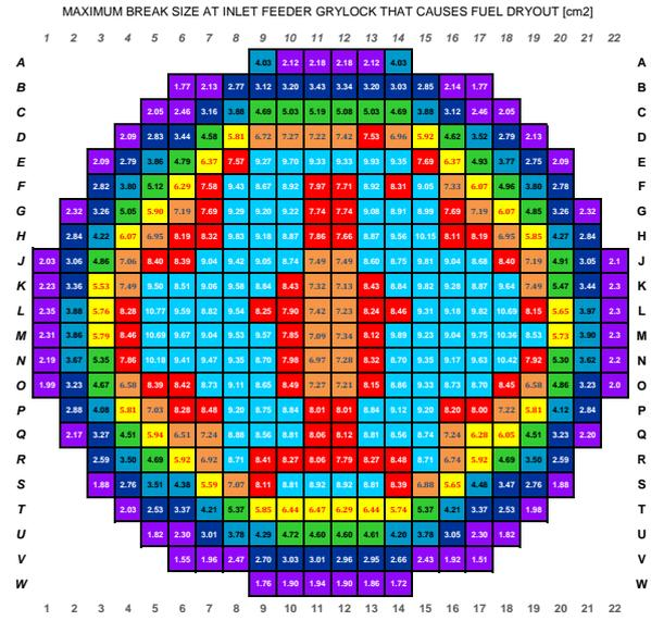
Fig. 9. Maximum break size at inlet feeder gray-lock that causes fuel dry-out [cm<sup>2</sup>]
