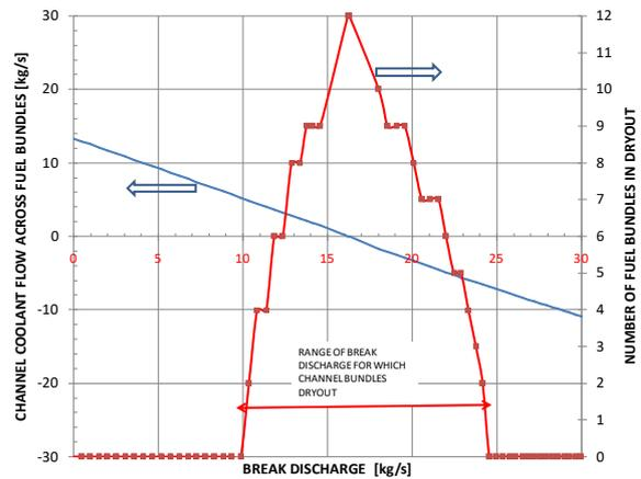
Fig. 5. Range of break discharges that cause a bundle to dry-out downstream of the break
