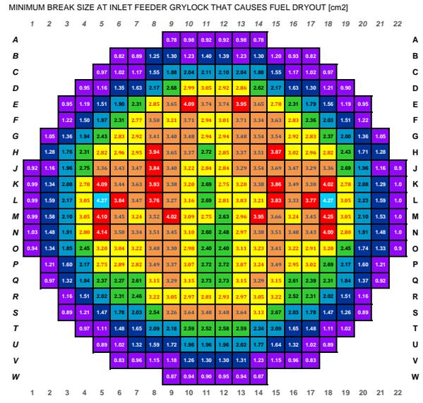
Fig. 8. Minimum break size at inlet feeder gray-lock that causes fuel dry-out [cm<sup>2</sup>]
