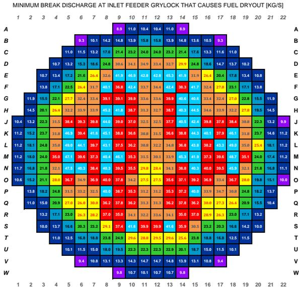
Fig. 6. Minimum break discharge at inlet feeder gray-lock that causes fuel dry-out [kg/s]
