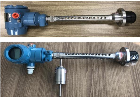
Fig. 1. The prototype of newly developed temperature compensated type pressure transmitter set: For system pressure measurement (up), for temperature compensation (down)
