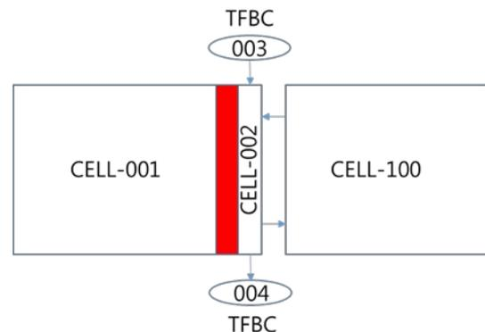
Fig. 1. Containment cooling analysis nodalization.
