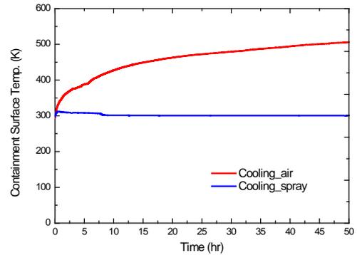
Fig. 4. Comparison for temperature change of containment surface according to cooling method during decay heat.
