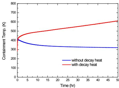
Fig. 2. Comparison for temperature change of containment inside with decay heat generation.
