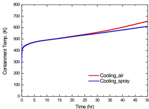
Fig. 3. Comparison for temperature change of containment inside according to cooling method during decay heat.
