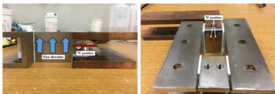
Fig. 4. Picture of test section with TCs location (left: side view, right: top view)
