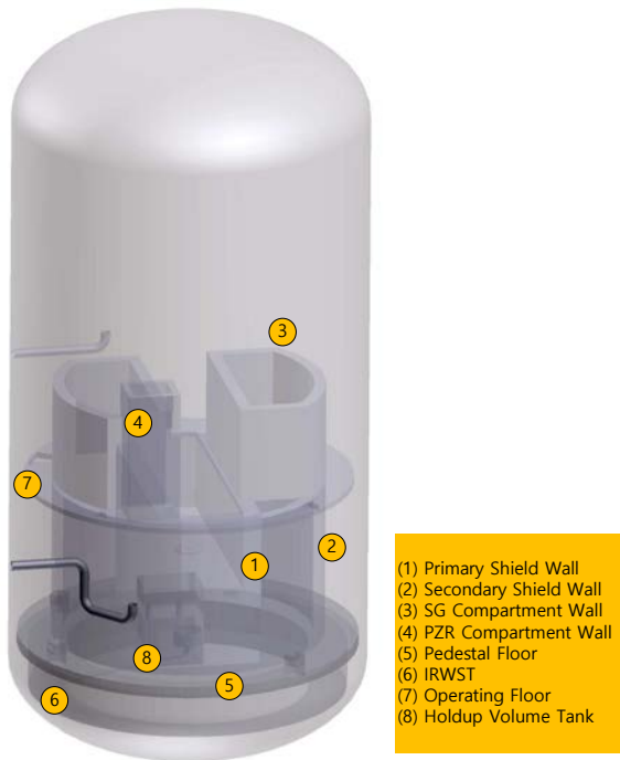
Fig. 2 Internal structure of the containment simulation vessel
