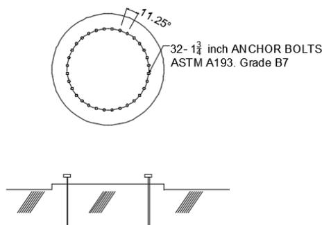
Figure 3. Schematic arrangement of anchor bolts
