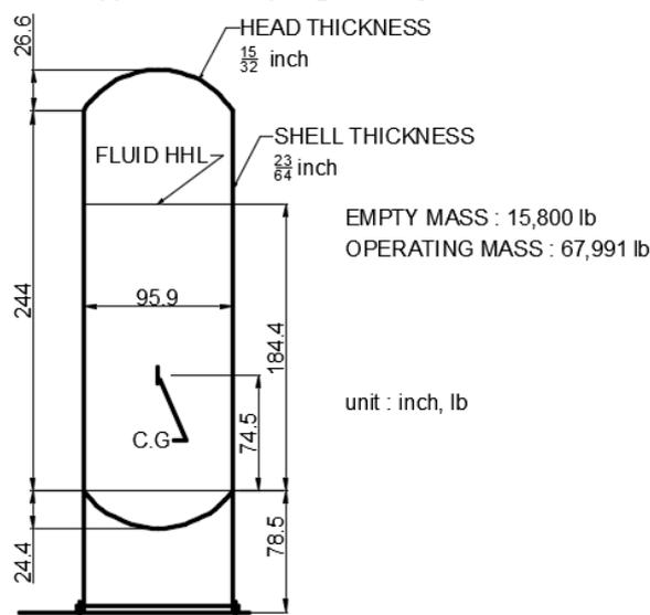
Figure 2. Outline of vertical elevated tanks
