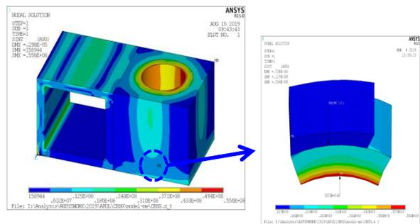
Fig. 8. Structural integrity evaluation section of CBSG module cell
