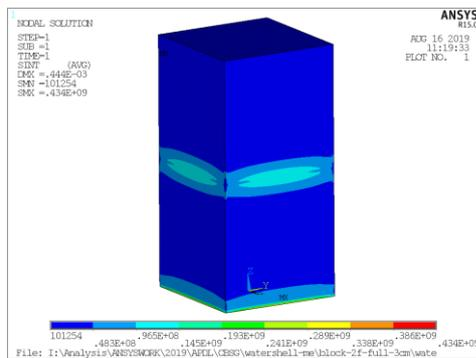
Fig. 9. Stress distribution of the water connection header for the pressure
