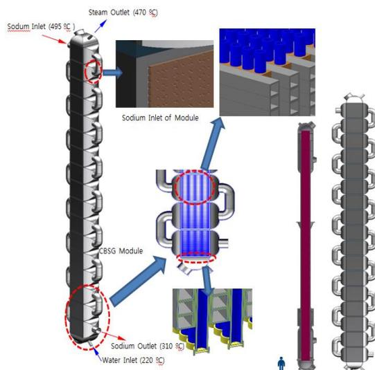
Fig. 1. Preliminary conceptual drawing of the CBSG designed by KAERI
