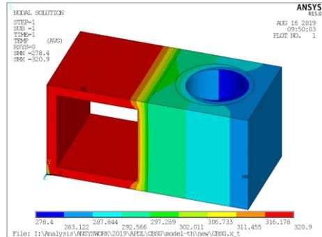
Fig. 6. Temperature distribution of the CBSG module cell for the thermal load
