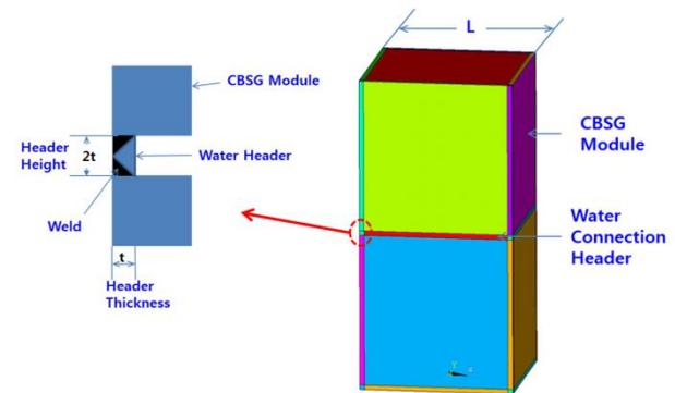
Fig. 11. Design configuration of the water connection header
