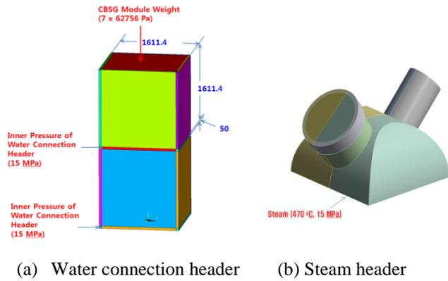
Fig. 4. Loading condition of water connection header and steam header
