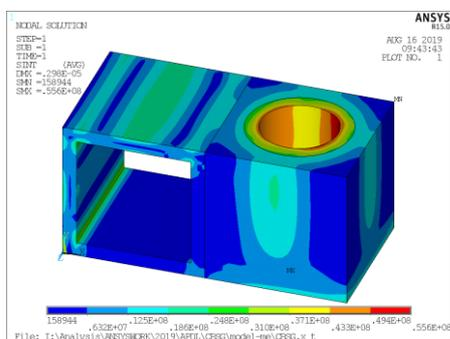
Fig. 5. Stress distribution of the CBSG module cell for the pressure
