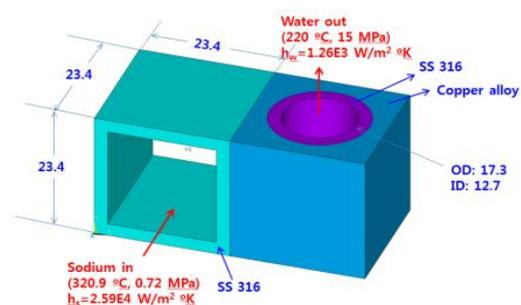
Fig. 3. Loading condition of CBSG Module cell
