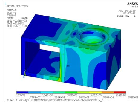
Fig. 7. Stress distribution of the CBSG module cell for the thermal load
