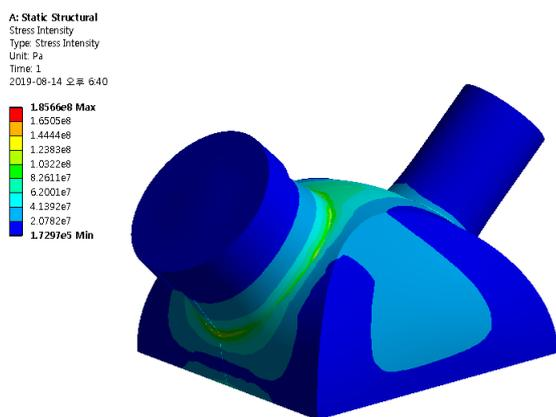
Fig. 10. Stress distribution of the steam header for the pressure
