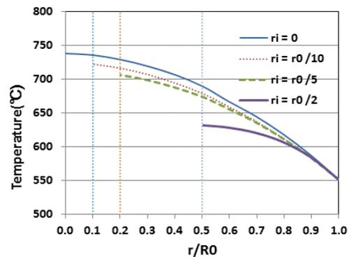
Fig.2. Annular fuel slug radial temperature distribution according to inner radius (helium gap, burnup : 1.3 at.%)
