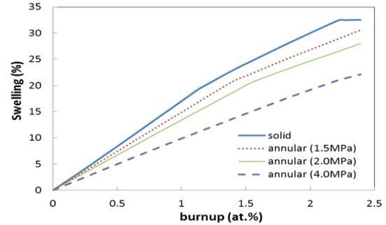
Fig.3. Comparison of the swelling of the annular fuel according to the hydrostatic stress.
