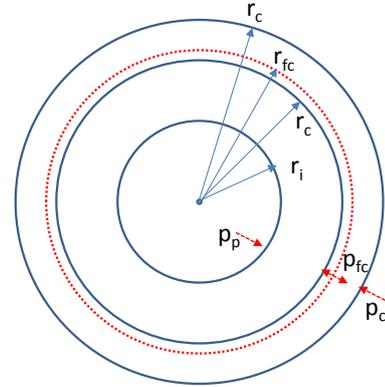
Fig. 1. Fuel and cladding geometry & elastic fuel-cladding mechanical interaction schematic
