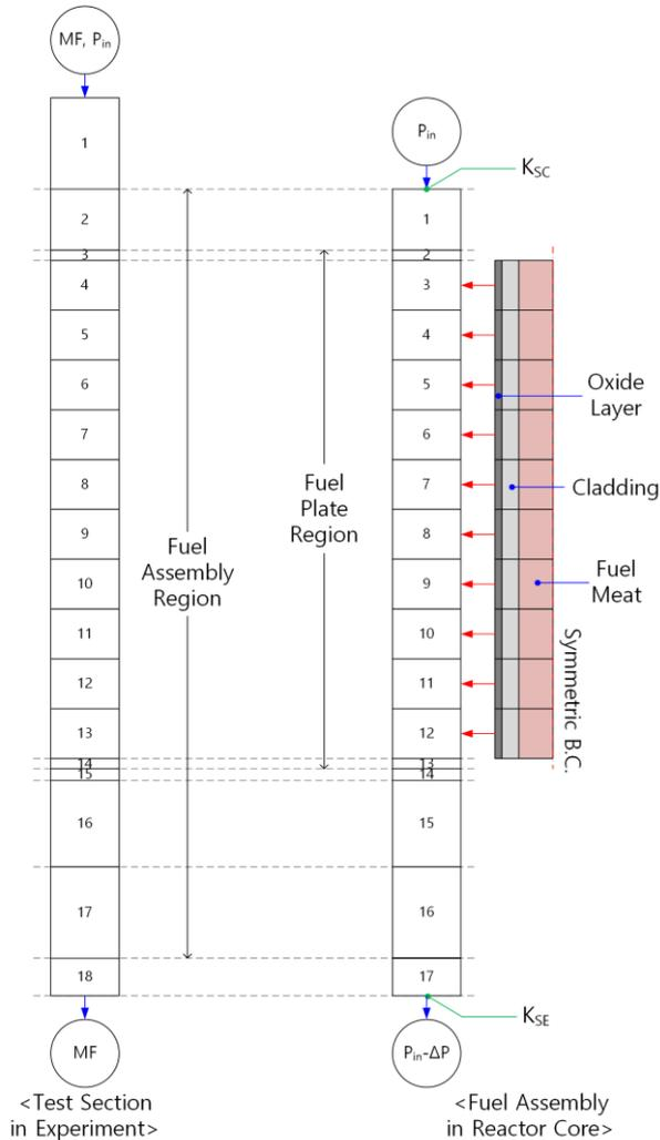
Fig. 1. Discretized Geometry for CORAL Simulation.
