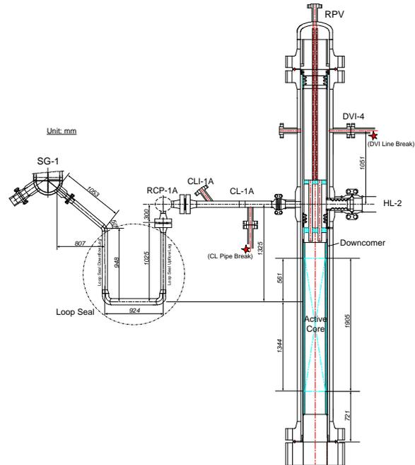
Fig. 1 Schematic arrangement of loop seal in ATLAS facility
