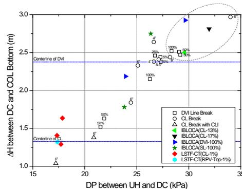
Fig. 4 Comparison of pressure difference (UH-DC) vs. water level difference (DC-COL)
