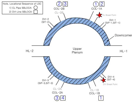
Fig. 5 Sequence of LSCs in CL pipe and DVI line SBLOCAs
