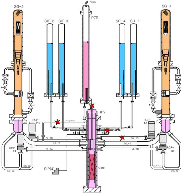
Fig. 2 Break locations for SBLOCA and SBO-related tests in ATLAS facility
