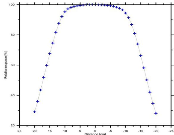
Fig. 2. Beam profile of G10 gamma beam irradiator
