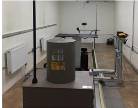
Fig. 1.  $^{137}\text{Cs}$  source with G10 gamma beam irradiator.
