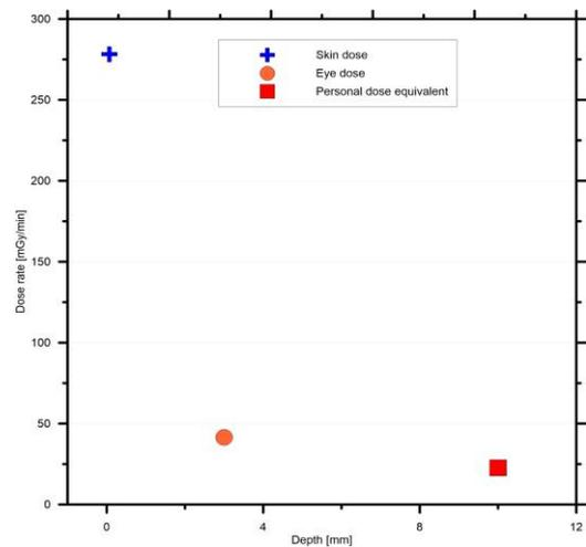
Fig. 5. Dose rate as a function of depth from  $^{137}\text{Cs}$  source.
