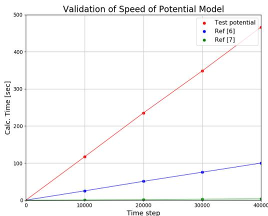
Fig. 4. Comparison of calculation cost of the developed potential model and two existing potential models [6], [7].
