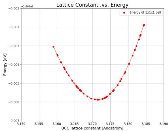
Fig 1. Potential energy calculated by the developed potential model as a function of lattice constant of bcc-W crystal.
