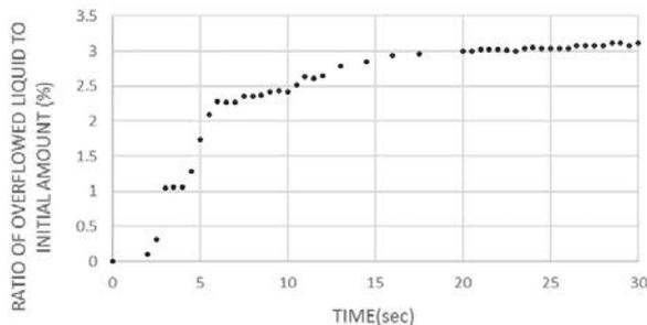
Fig. 4. Ratio of overflowed liquid to initial amount under seismic excitation.
