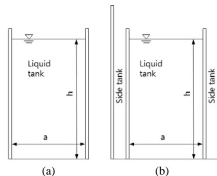
Fig. 1. Typical geometry of a partially filled rectangular container without side tank (a) and with side tank (b).
