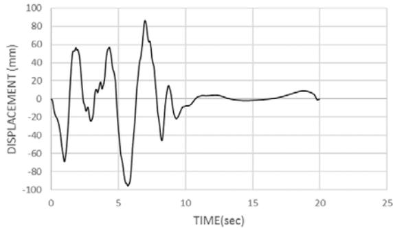
Fig. 2. Displacement-time history of seismic excitation.
