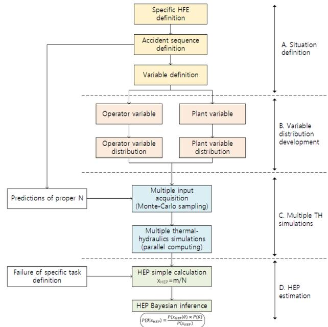
Fig. 1. Overall flowchart of the HuTEC method (human error probability estimation through TH simulation with exhaustive conditions)
