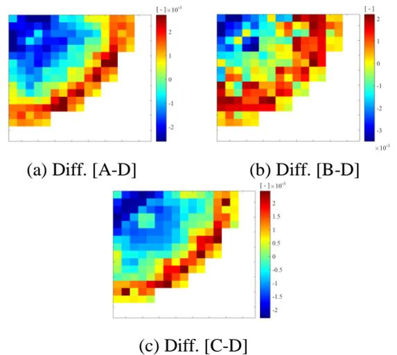
Figure 3. Difference of radial power distribution at EOC (13.8 GWd/MTU)
