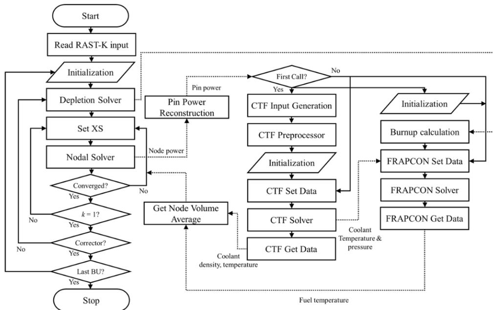
Figure 1. Flowchart of coupled calculation
