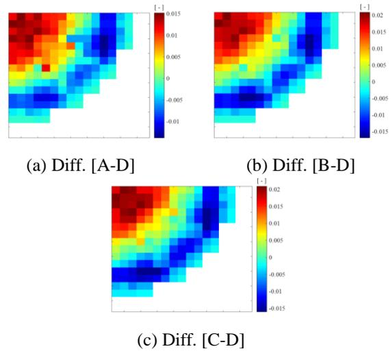
Figure 2. Difference of radial power distribution at BOC (0.0 GWd/MTU)
