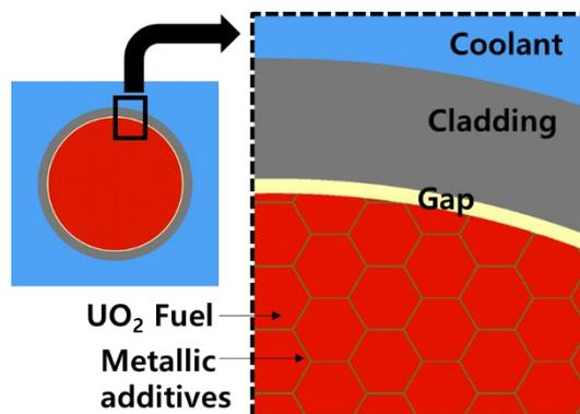
Fig. 2. Heterogeneous ATF microcell structure
