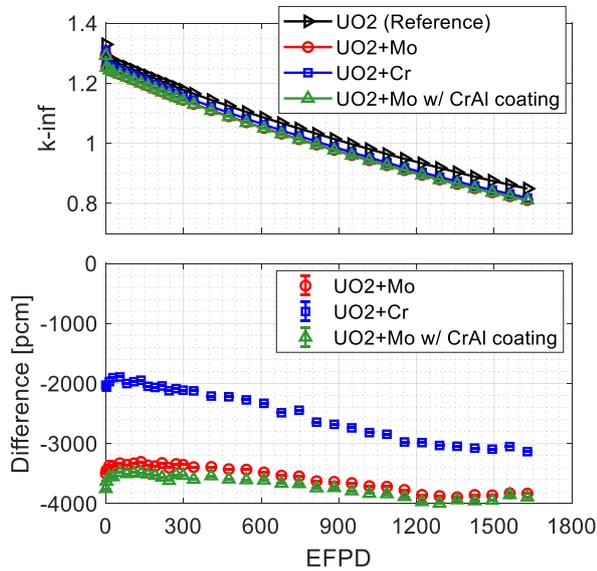
Fig. 3. Comparison of infinite multiplication factors
