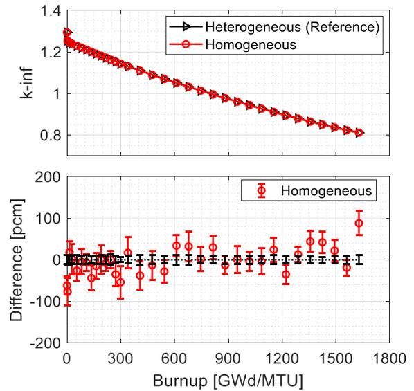
Fig. 6.  $k$ -inf comparison depends on heterogeneity of  $UO_2+Mo$  case
