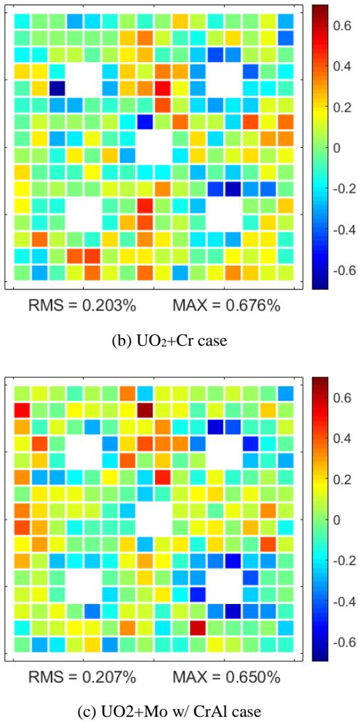
Fig. 5. Relative difference of pin power distribution at BOC
