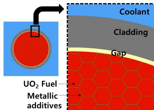
Fig. 2. Heterogeneous ATF microcell structure
