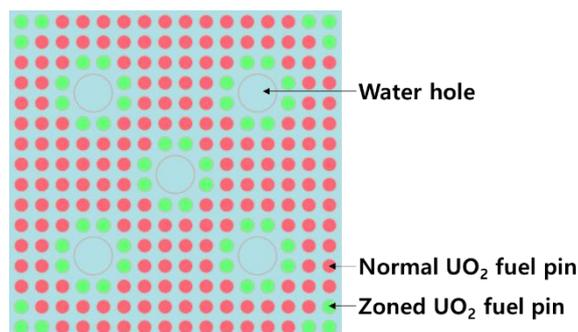
Fig. 1. PLUS7 16×16 fuel assembly model
