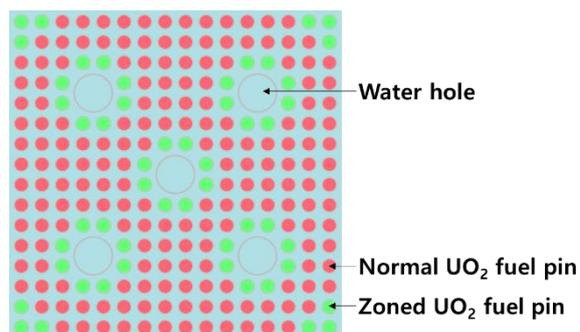
Fig. 1. PLUS7 16×16 fuel assembly model
