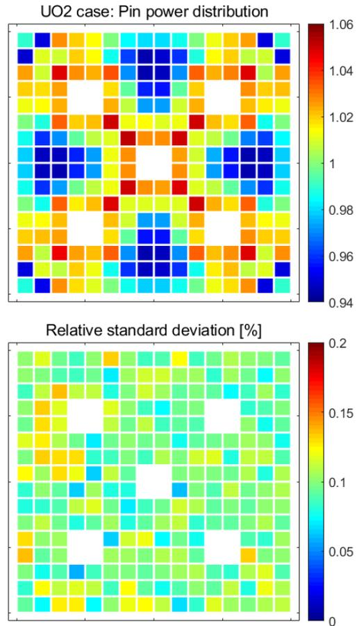
Fig. 4. Normalized pin power distribution and relative standard deviation of  $\text{UO}_2$  case at BOC
