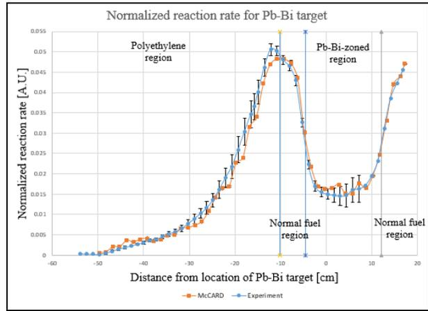
Fig. 10. Comparison between McCARD calculation and experimental results of  $^{115}\text{In}(n,\gamma)^{116m}\text{In}$  reaction rate distributions for Case II-6
