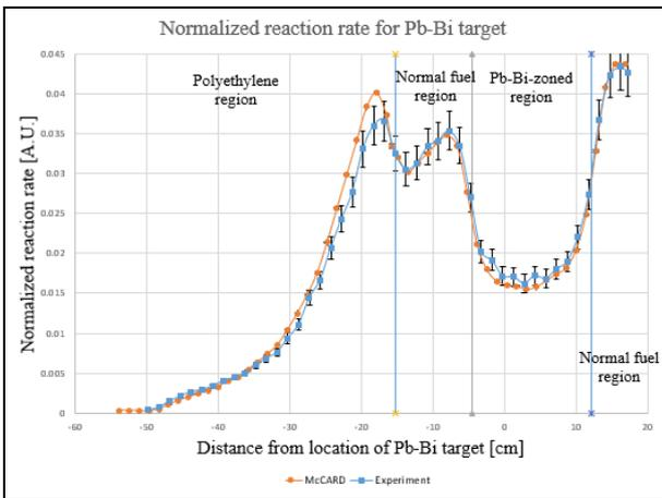
Fig. 8. Comparison between McCARD calculation and experimental results of  $^{115}\text{In}(n,\gamma)^{116m}\text{In}$  reaction rate distributions for Case II-4
