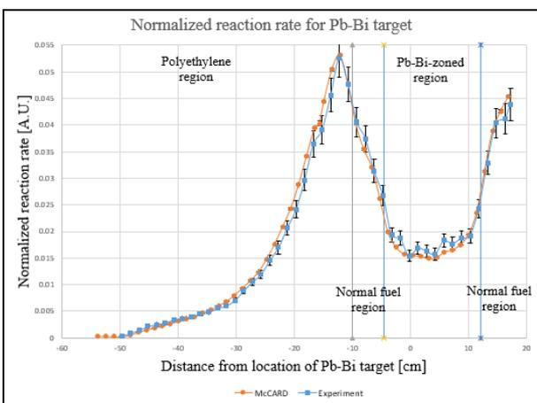
Fig. 9. Comparison between McCARD calculation and experimental results of  $^{115}\text{In}(n,\gamma)^{116m}\text{In}$  reaction rate distributions for Case II-5
