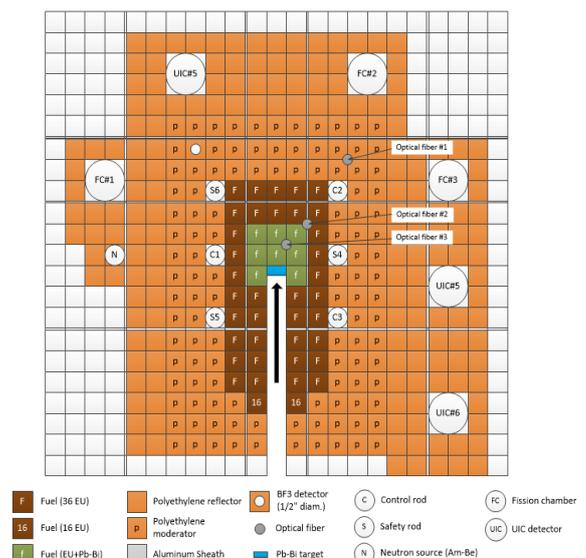
Fig. 4. Core configuration of ADS with 100 MeV protons
