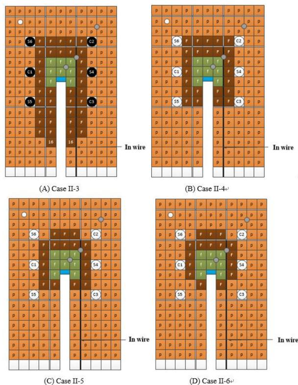
Fig. 6. Subcritical core configurations
