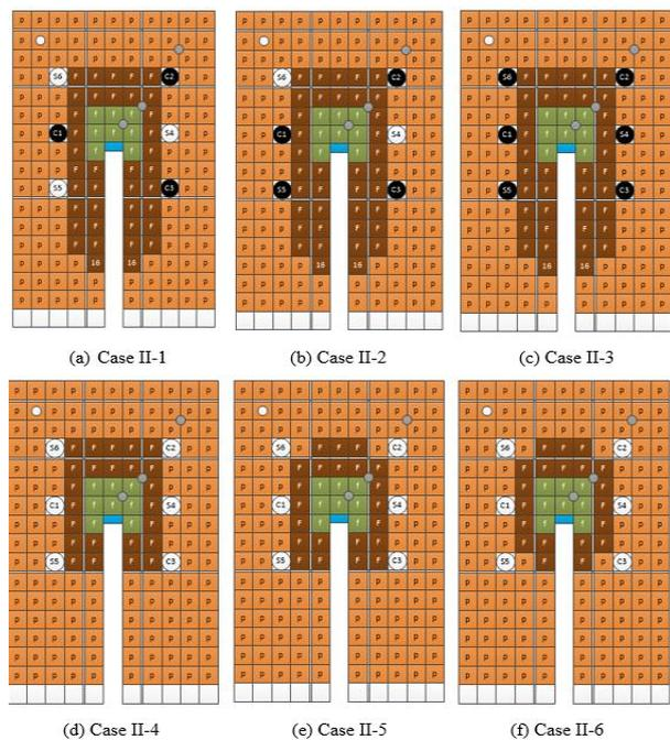
Fig. 5. Subcritical core configurations
