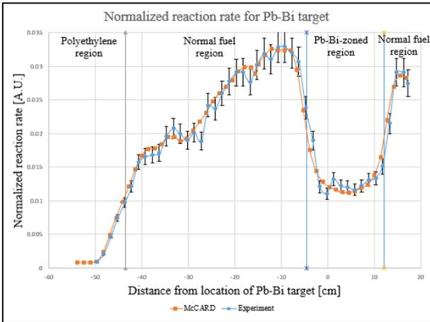
Fig. 7. Comparison between McCARD calculation and experimental results of  $^{115}\text{In}(n,\gamma)^{116m}\text{In}$  reaction rate distributions for Case II-3
