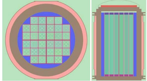
Fig. 1. The horizontal and vertical cross-sectional view of TN-32 cask.
