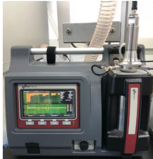
Fig. 1. The real-time aerodynamic diameter (range: 6 \text{ nm} - 10 \mu\text{m} ) distribution was measured by the HR-ELPI+ (Dekati).
