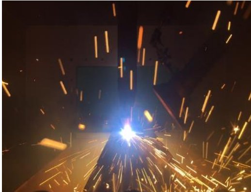
Fig. 3. The stainless-steel cutting with the plasma arc torch
