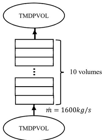
Fig. 1. MARS input geometry
