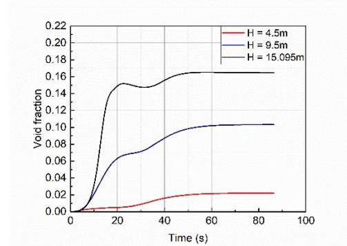
Fig. 2. Void fraction in the riser with time from MARS calculations at different elevations.
