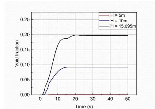
Fig. 3. Void fraction in the riser with time from MATLAB calculations at different elevations.
