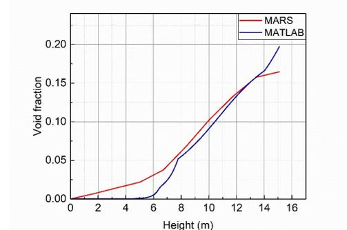
Fig. 4. Converged void fraction distribution in riser from MARS and MATLAB calculations.
