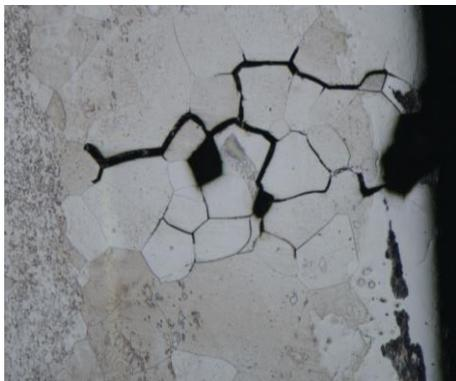
Fig. 3. Microstructure of crack on Fe-12Cr-2Si
