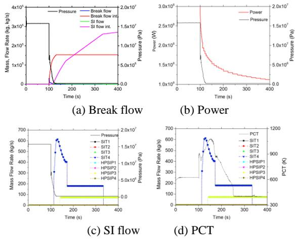
Fig. 3. Primary Physical Properties during LBLOCA Simulation
