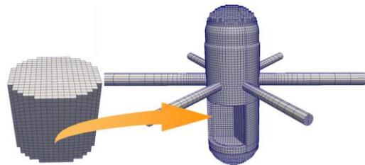
Fig. 1. Three-dimensional Mesh Model for APR1400 LBLOCA Analysis
