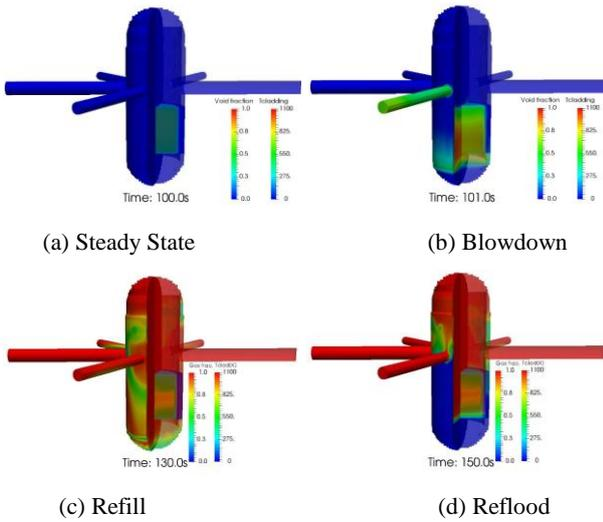
Fig. 2. Three-dimensional Contours Obtained from LBLOCA Simulation
