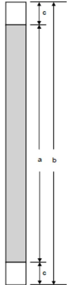
a = 350.52 cm  $\text{UO}_2\text{-Gd}_2\text{O}_3$  Pellets
