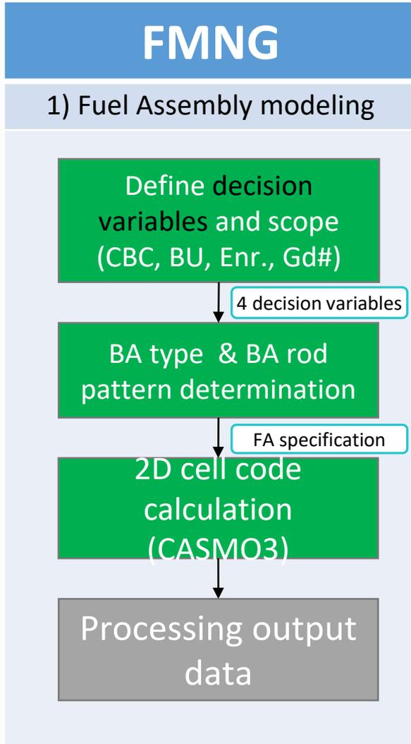
Four parameters are taken into consideration in constructing the FMNG:
