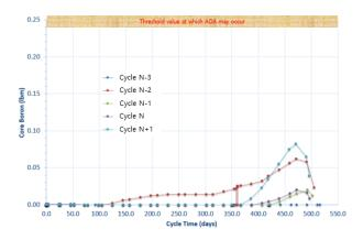
Fig. 2. Core boron mass with measured flow rate
