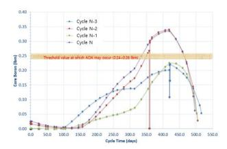
Fig. 3. Core boron mass with 5% reduced measured flow rate
