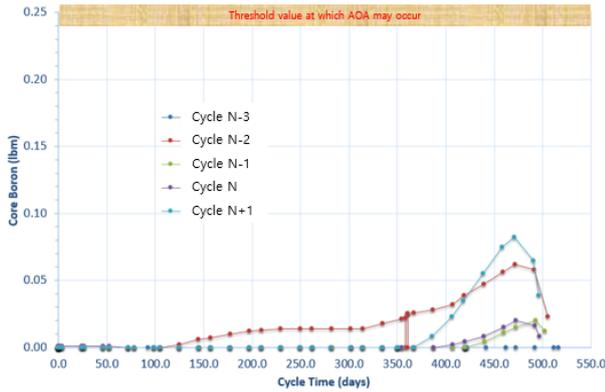
Fig. 2. Core boron mass with measured flow rate
