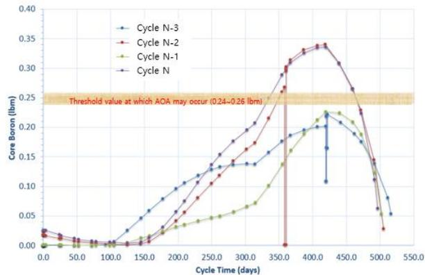
Fig. 3. Core boron mass with 5% reduced measured flow rate
