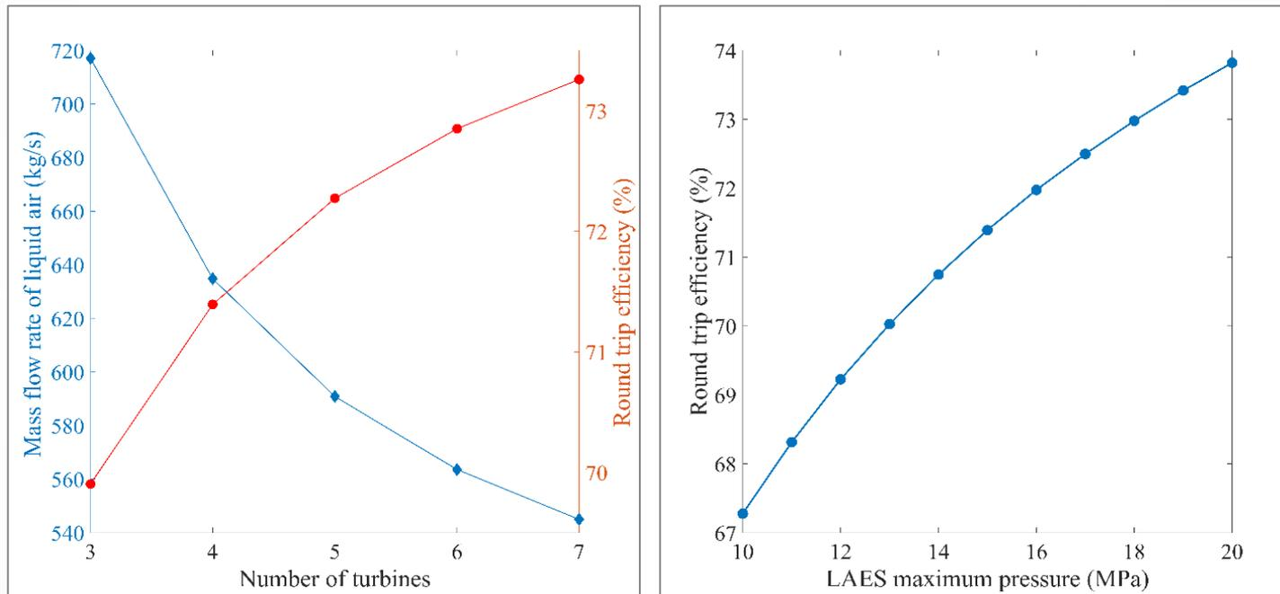
Fig. Performance of integrated system w.r.t. number of turbines (left) and maximum pressure (right)
