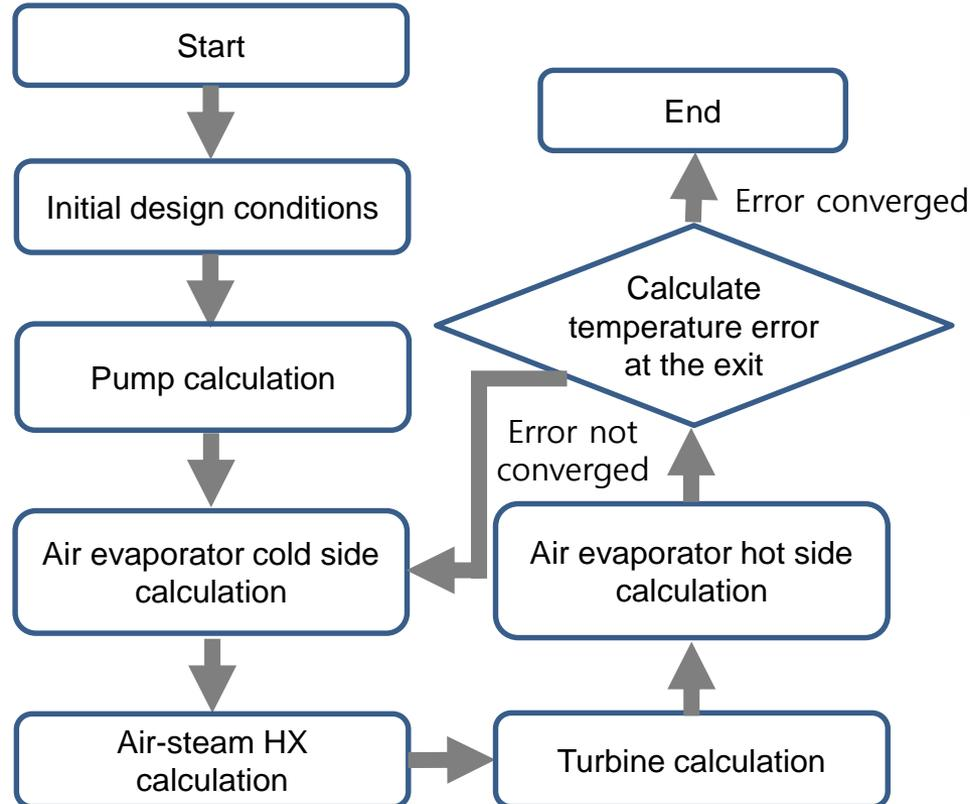
Fig. KAIST-CCD code algorithm for NPP-LAES design
