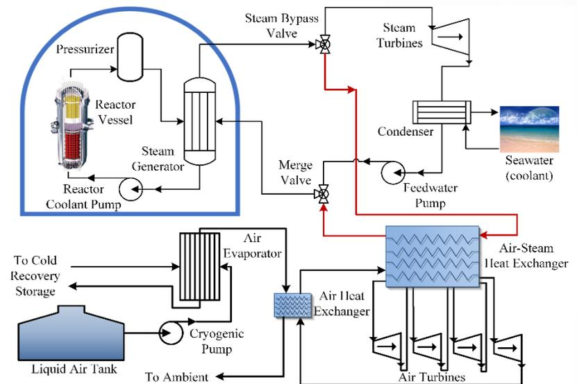
Fig. Schematic of APR1400 integrating the LAES system (discharge cycle)
