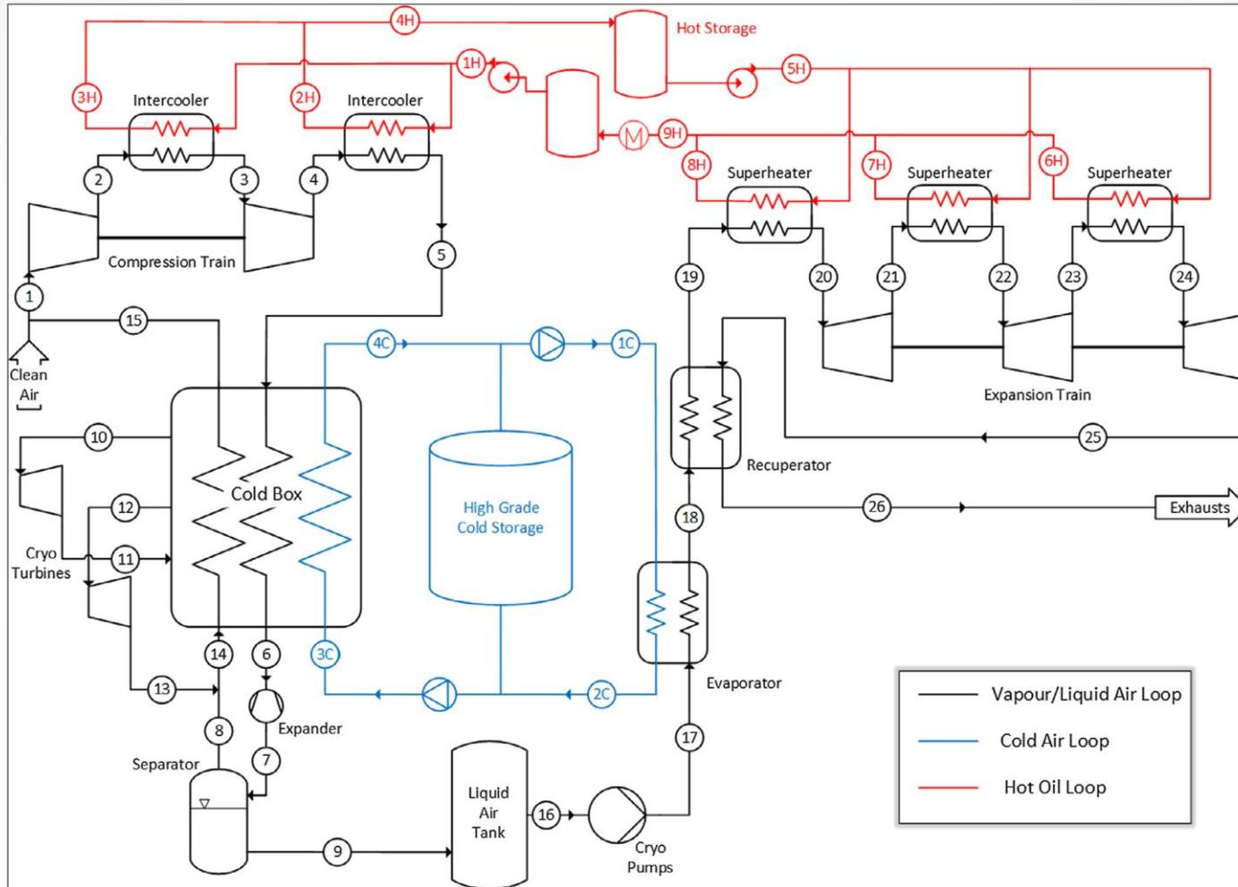
LAES principle: Charge (liquefaction) – storage (liquid air, thermal storage) – discharge (open Rankine cycle)
