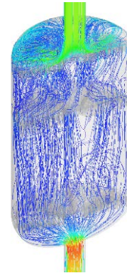
Fig. 2. 3D massless particle contour using DPM method
