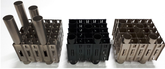
Fig. 3. Nuclear fuel support grids (Inconel 718, PBF)
