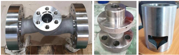
Fig. 4. Body, bonnet, cage parts for nuclear safety class 1 3-in. valve. (SUS 316, BJ aided casting)
