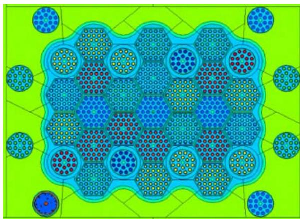
Fig. 1 Configuration of OR irradiation hole in HANARO
