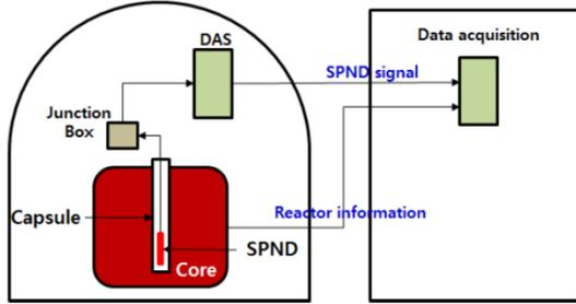
Fig. 3 Overview of SPND signal acquisition system
