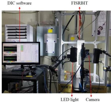
Fig. 1. Photograph of the 'FISRBIT' facility with the 3D-DIC system
