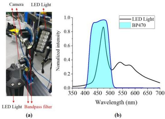
Fig. 2. (a) photograph of bandpass filter mounted on the 3D-DIC system and (b) spectral properties of LED light and BP470 filter.
