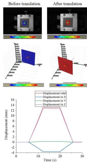
Fig. 4. Experimental validation results from the 3D-DIC system before and after translation.
