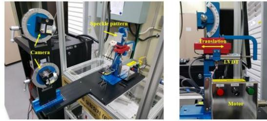
Fig. 3. Custom designed validation device for the 3D-DIC system
