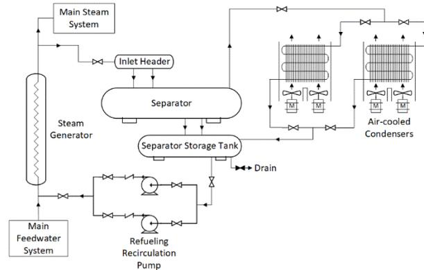
Fig. 1. Schematic Diagram of the PGSFR RDHRS
