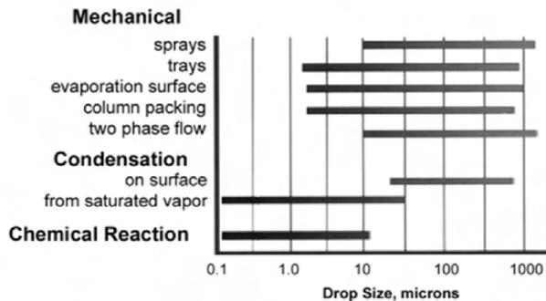
Fig. 3. Typical Particle Size Distribution Ranges from Entrainment caused by Various Mechanisms [1]
