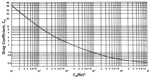
Fig. 2. Drag Coefficient of Rigid Spheres [1]
