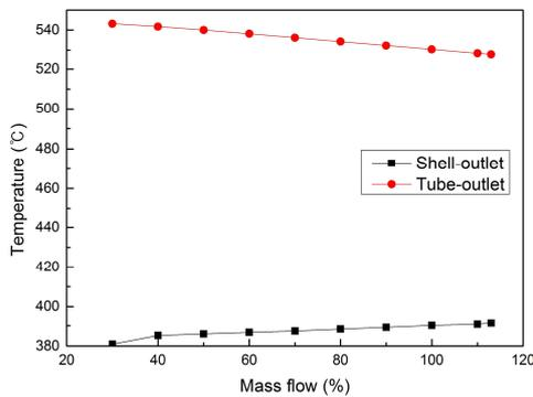
Fig. 5. IHX outlet temperature
