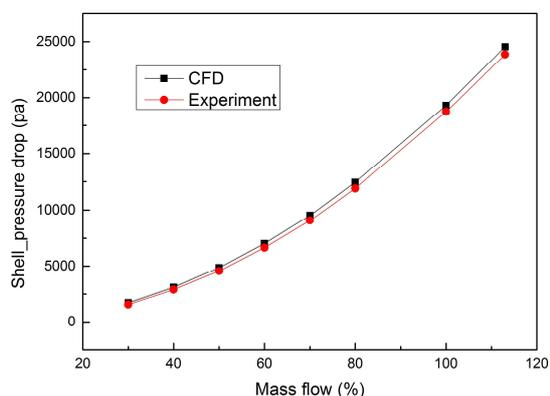
Fig. 3. IHX shell side pressure drop with mass flowrate variation
