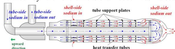
Fig. 1. Schematic view of IHX
