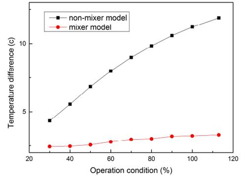
Fig. 6. IHX tube outlet temperature difference between inside and outside wall
