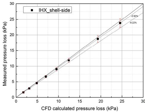
Fig. 4. IHX shell side pressure drop comparison CFD result and Measured
