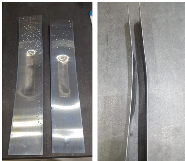
Fig. 4. An image of a hot-rolled target after thermal annealing
