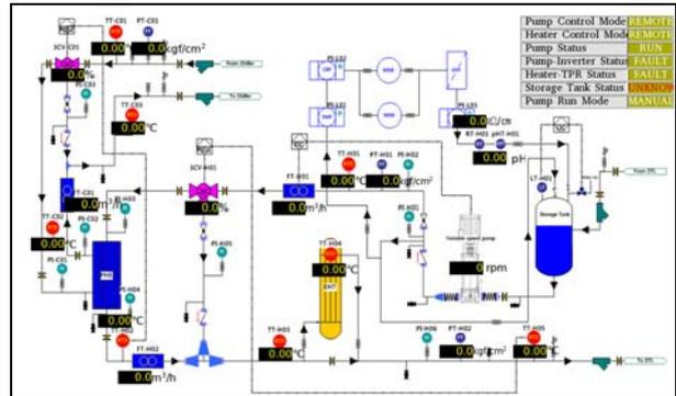
Fig. 2. RCCS's piping and instrument diagram [3]
