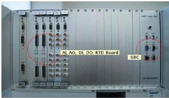
Figure 4. The control I/O unit
