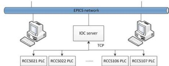
Figure 6. EPICS IOC Server Block Diagram
