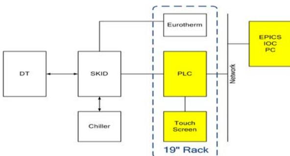
Figure 5. RCCS 21,22 Control Panel Block Diagram.
