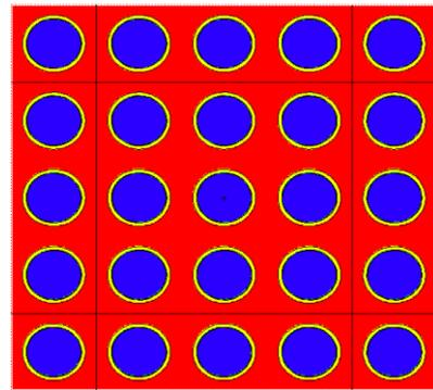
Fig. 1. Typical 5 × 5 cross-sectional drawing for PLUS7™ fuel rod bowing calculation
