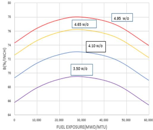
Fig. 3. Linear heat rate augmentation coefficient vs. fuel burnup
