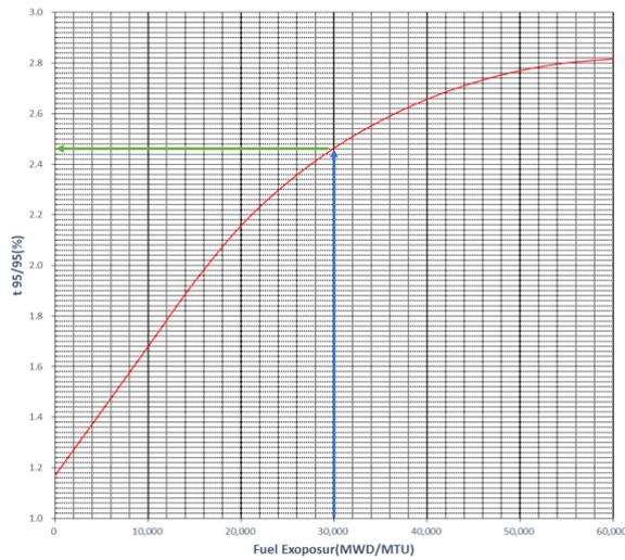
Fig. 7. Rod bow augmentation factor for PLUS7™ fuel
