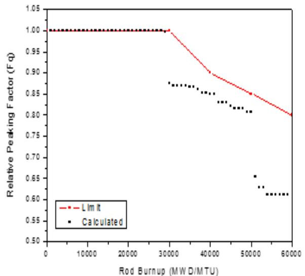
Fig. 6. Peak rod power burndown curve of PLUS7™ fuel
