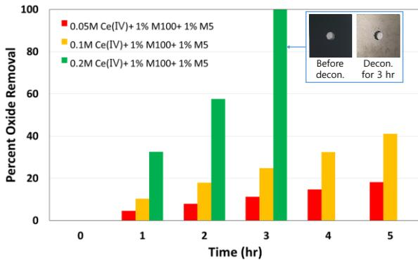
Fig. 2. FeCr<sub>2</sub>O<sub>4</sub> Oxide Film Removal Performance Using Oxidative Decontamination Foams.
