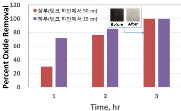
Fig. 3. Bench Scale Oxide Removal Performance Using Oxidative Decontamination Foams.
