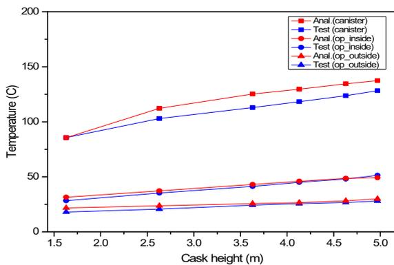
Fig.4. Thermal test results for prototype cask and scale model with various heat fluxes
