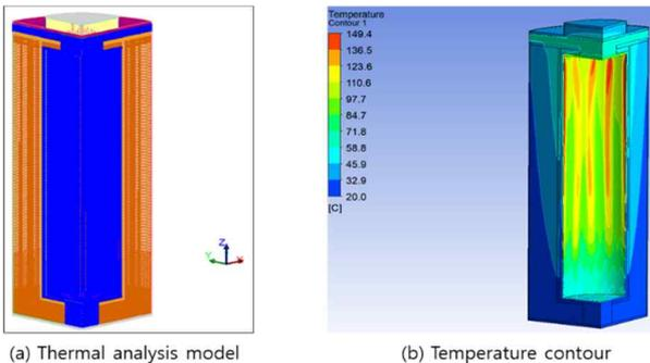
Fig. 1. Thermal analysis model and temperature contour
