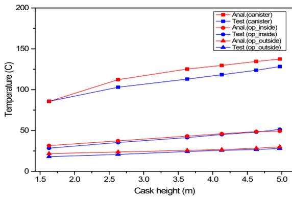
Fig.3. Temperature profiles between thermal test and analysis for prototype cask
